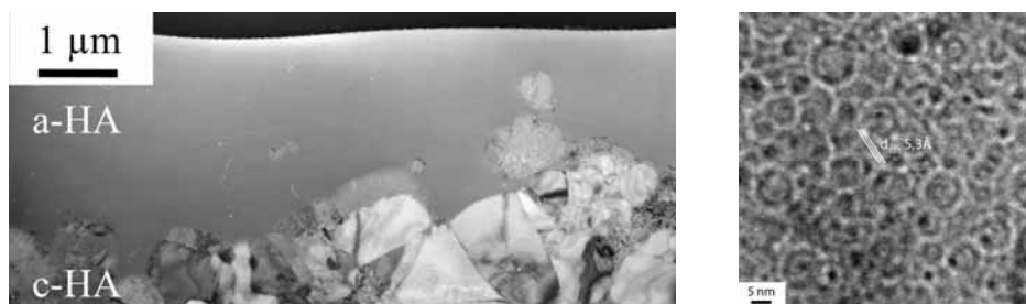
Figure 17: Left) Bright field TEM micrograph of the sample, the outermost layer is amorphous while the subsurface layer is crystalline. Right) Hydroxyapatite phase in the crystalline part is identified by HRTEM.
