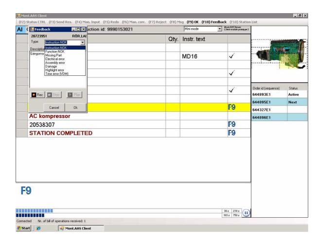
Figure 5: The feedback/deviations reporting interface integrated with the assembly instructions interface in the mini mode.
