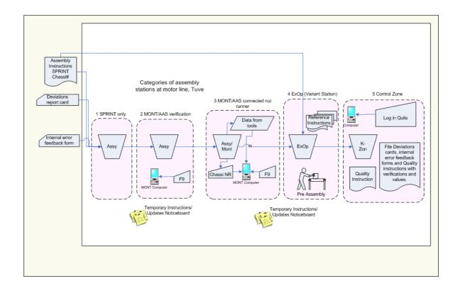
Figure 3: Information environment at the motor assembly line
