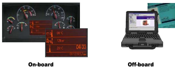
Figure 3.1: Examples of the two types of diagnostics systems, where the dashboard represents the on-board system and the laptop computer, with VCADS Pro software, represent the off-board system.
