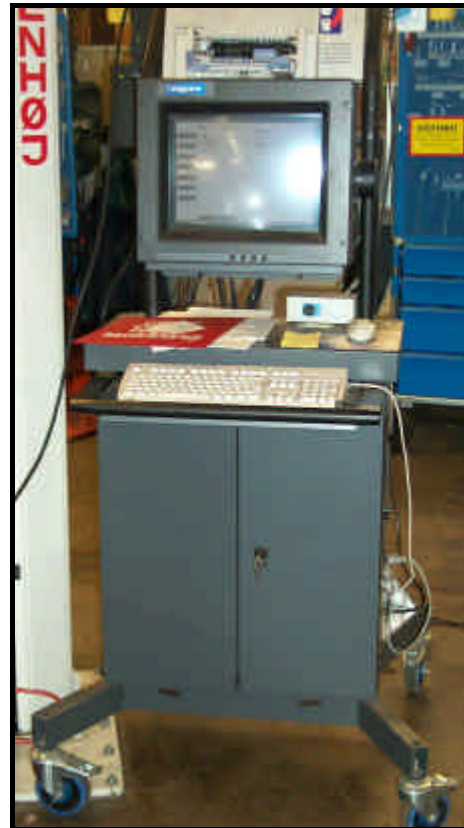
Figure 3 – The VADIS cart. it consist of a standard PC wrapped in a metal case. It is equipped with touch screen, mouse
