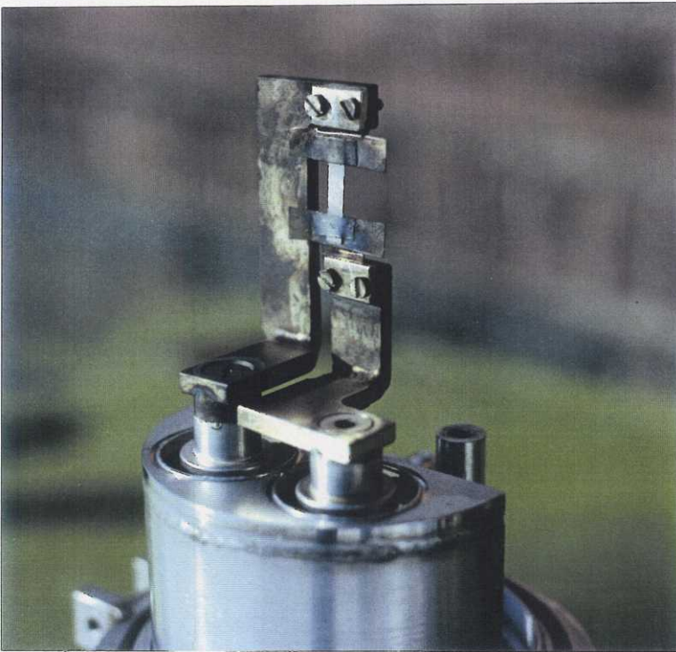
Fig. 8. The emitter assembly with a mounted 20 mm long, 5 mm high and 0.5 mm thick Mo emitter foil. The round part is the interface between the vacuum chamber and the air. One of the two studs for an extra electrode can be seen behind the emitter.
