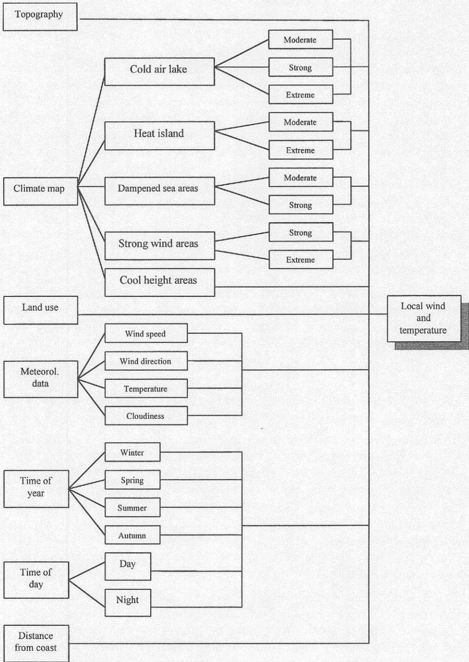
**Figure 7.** Descriptive diagram showing input parameters to the local climate model.
