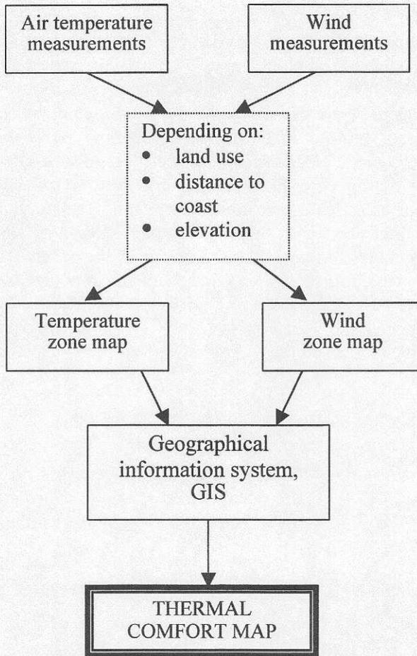
*Figure 8. Flow diagram showing the basic steps of the human comfort model for assessment of the thermal component.*
