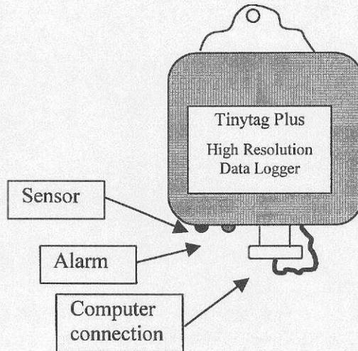
**Figure 5.** Photograph showing the Tiny-logger and radiation shield (a) and a graphic illustration of the Tiny-logger (b).
