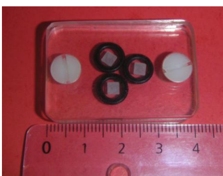
Figure 7.5. The plexiglass holder containing 3 TLD's.
