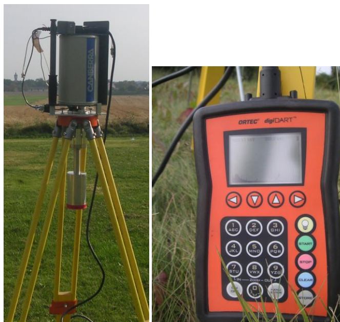
Figure 7.3. The HPGe detector and the measurement setup used in the in situ measurements.
