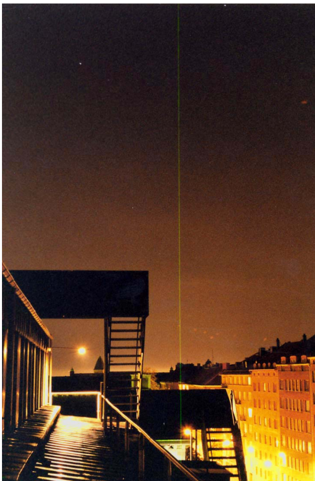
Fig. 6 A photograph showing the vertically directed green laser beam. At the bottom, the beam is exiting the lidar station booth hosting the telescope. The Göteborg city centre is in the background. (photo: Frans Olofson, 2004)
