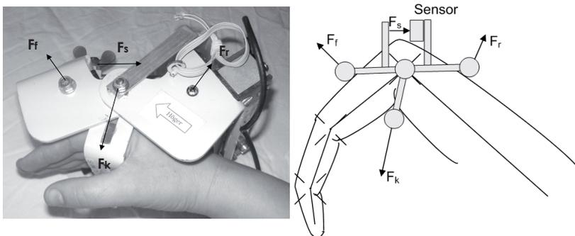
**Figure 10.** The forces  $F_k$  (force from the applied load),  $F_s$  (force on the sensor),  $F_f$  (force generated by the fingers under full extension),  $F_r$  (reaction force) are derived from MCP joint movement.
