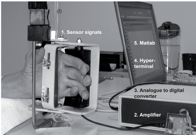
**Figure 12.** This picture shows one of the RA patients using the new extension force measurement device. The sensor signals (1) are transmitted by an amplifier (2) to a computer board with an analogue-to-digital converter (3) which is connected to a hyper terminal (4) on the computer. The measurements are evaluated in Matlab™ (5). The device is suspended on a metal wire with a nylon thread (I) to eliminate reaction forces from the hand and wrist during the measurements.
