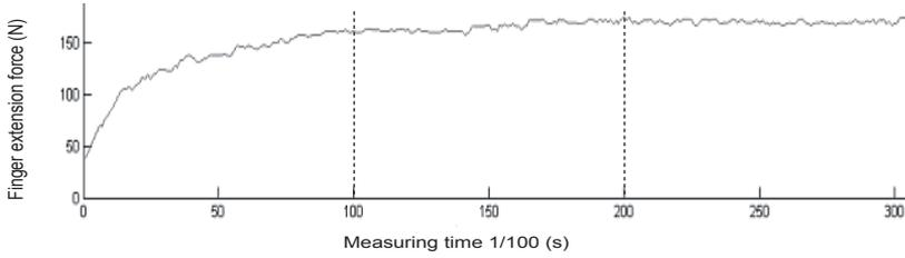
**Figure 16.** Force plot from whole hand measurement. The x-axis shows the time, in 1/100 second increments. The mean value between 100 and 200 is taken as the measured force value. The measurement results can be presented in graphs, on a computer screen or printed on paper, showing the mean, maximal forces and continuous force over the measured time.
