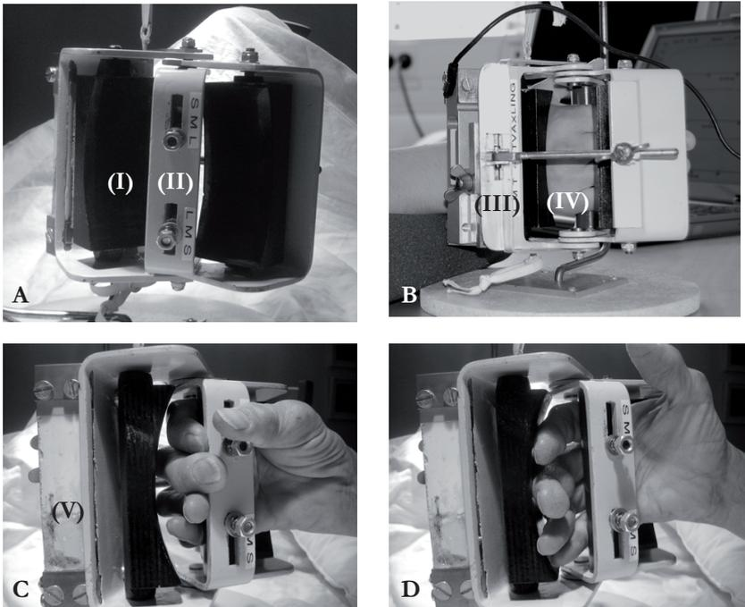
**Figure 11.** (A) Front view of the extension force measuring device, showing the hand pad (I), and the size adjustment control for hand size (II). (B) The rear view of the extension device, showing the gear mechanism (III), and the position for the MCP-joints (IV). (C) illustrates the sensor (V) and an RA patient using EX-it. (D) illustrates finger force measurements on an RA patient.
