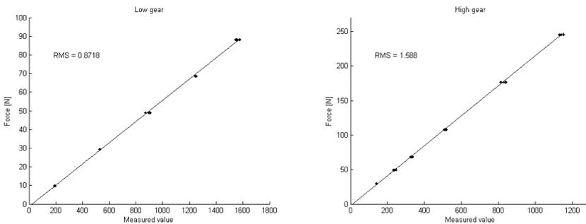
**Figure 15.** Validation of the low force interval, 0–95 N, left (RMS = 0.87 N), and the high force interval 0–385 N, right (RMS = 1.59N) the vertical axis shows applied load and the horizontal axis shows the digital value from the sensor.
