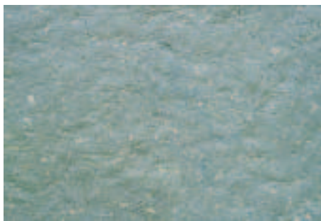
Figure 8. Paper-composite porcelain tile. Produced by the hand-press casting method with MCP 3 and fired at a temperature of 1300°C. No glaze was applied. Many fibre forms were seen on the surface of the tile.
