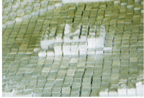
Figure 2. Wall decoration tile work. This was produced by the slip casting method with white porcelain.
