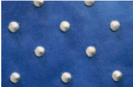
Figure 4. Paper-composite porcelain tile. This work is produced by the double-casting method (first slip casting and then press casting). The method was invented during the study of the paper-composite porcelain. The highest paper fibre content (the amount of paper in a slip was 90% by volume as 39.8% in weight) was used. The coloured paper-composite porcelain was mixed with cobalt mono-oxide. No glaze was applied, however the ashes from the paper gave it a natural glaze effect.
