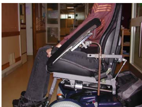
Figure 5. (a) The arm support attached to the electric power driven wheelchair. (b) Not only is the elbow motion restricted, the shoulder is also restricted from being adducted.
