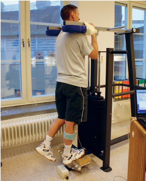
Figure 8. Weight machine used for the strength testing (concentric and eccentric-concentric heel-rises).
