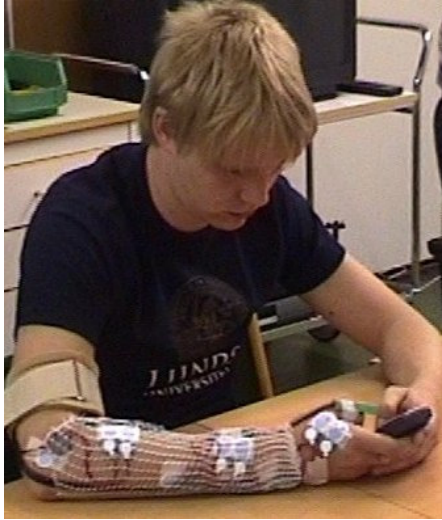
Figure 4 The position of the EMG electrodes during text entering on mobile phone in Paper III and IV .
