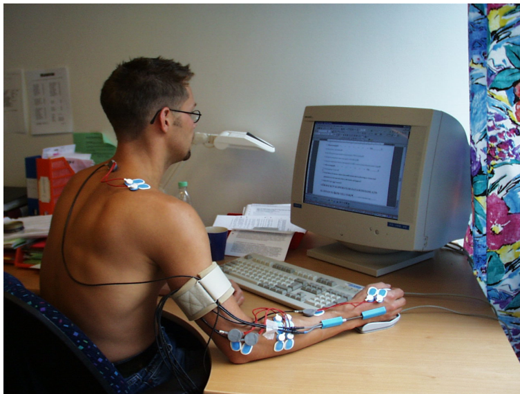
Figure 3 The position of the EMG electrodes and the electrogoniometer in work with the vertical mouse in Paper II .
