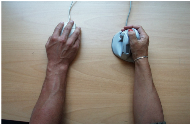
Figure 1 The traditional mouse with the pronated hand position to the left and the vertical mouse with the neutral hand position to the right. The main button of the vertical mouse is placed under the pad of the index (or middle) finger when gripping the mouse and you use the button by pushing it horizontally towards the mouse.
