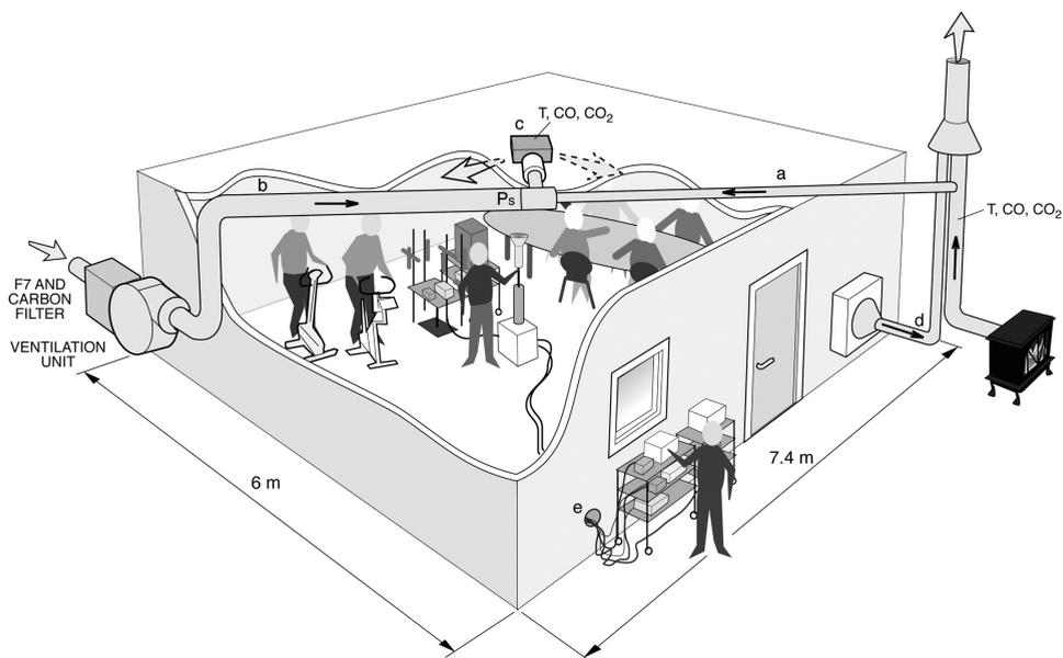
**Figure 3.4.** The chamber (dimensions of 7.4 m × 6 m × 2.9 m) used in **Paper IV**. Partial flow of flue gas (a), flow of filtered indoor air (b), supply of air terminal device (c), ventilation outlet (d), and connection hole for instruments (e).
