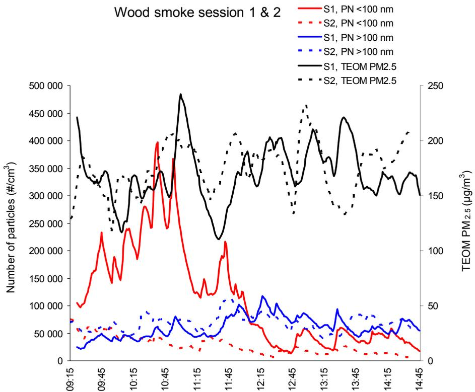
**Figure 4.9.** Particle number concentrations and particle mass ( $PM_{2.5}$ ), as measured online using an electric low-pressure impactor (ELPI) and a tapered element oscillating microbalance (TEOM), respectively, during 5.5 h in an exposure chamber with wood smoke
