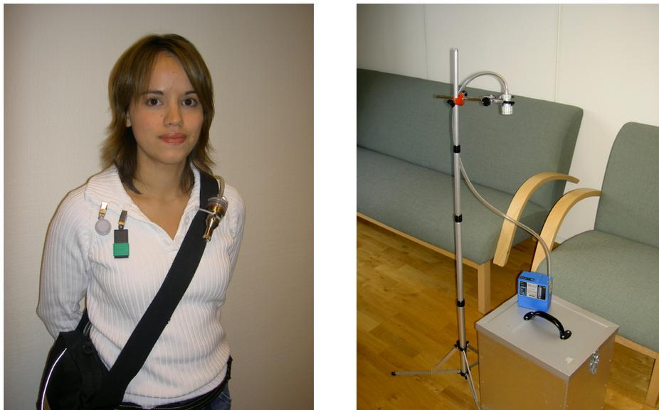
**Figure 3.3** The personal SKC and UMEEx samplers (left) and the indoor PAH sampling equipment (right).
