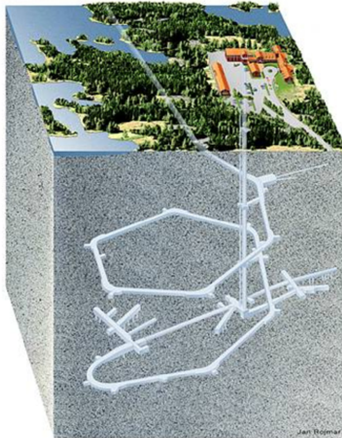
Figure 2 Schematic view of the field site Äspö hard rock laboratory, showing how the tunnel spirals down to a depth of approximately 450 m into the granitic rock. The artwork is provided by SKB (skb.se).
