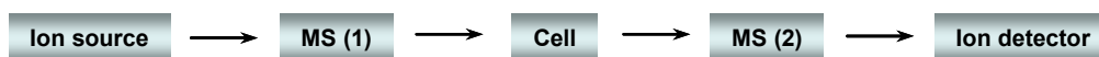
Figure 6. Diagrammatic outline of a system for MS/MS experiments. A collision cell is shown between the two mass spectrometer instruments.
