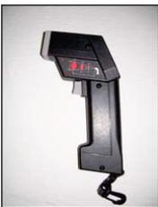
**Figure 1.** Raytec Raynger ST2L
