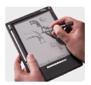
Figure 3. Handwriting on an iRex iLiad device with e-paper display [8]
