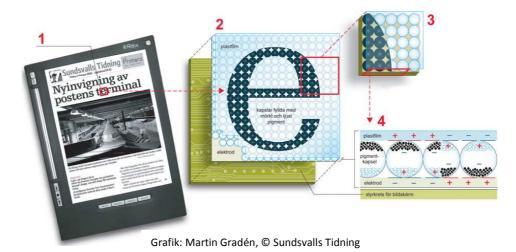
**Figure 1.** The principle of e-paper displays
