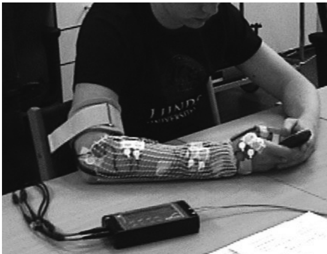
Figure 9. Subject entering a text message on a mobile phone. The picture shows the goniometer spanning the wrist joint and mounted on thumb, the EMG electrodes mounted on the hand and forearm, and the logger used to record and pass the data onto the PC.
