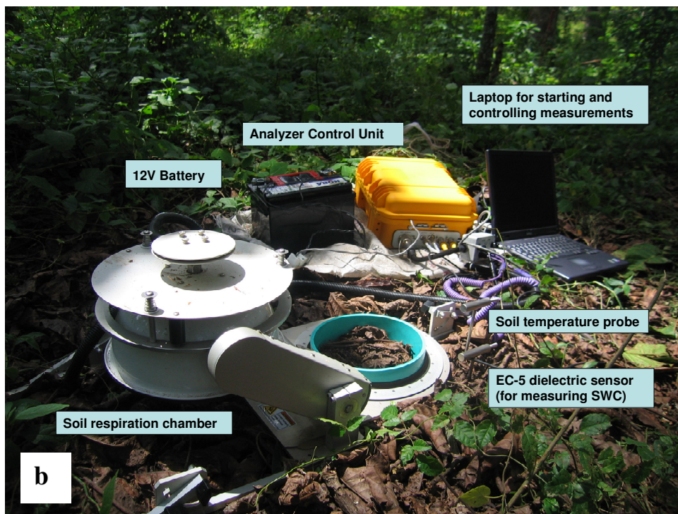
Figure 2. Measurement of soil CO 2 efflux in the field using the LI-6400 soil respiration system (a) and Diurnal soil CO 2 efflux measurement using the LI-8100 automated soil CO 2 flux system (b) ( Papers II, III, and IV ).
