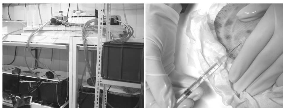
Figure 12. Within this thesis, long term water exposures have been performed using flow-through systems controlled by peristaltic pumps (left). For short exposures, intra peritoneal injection of medetomidine have been used (right).
