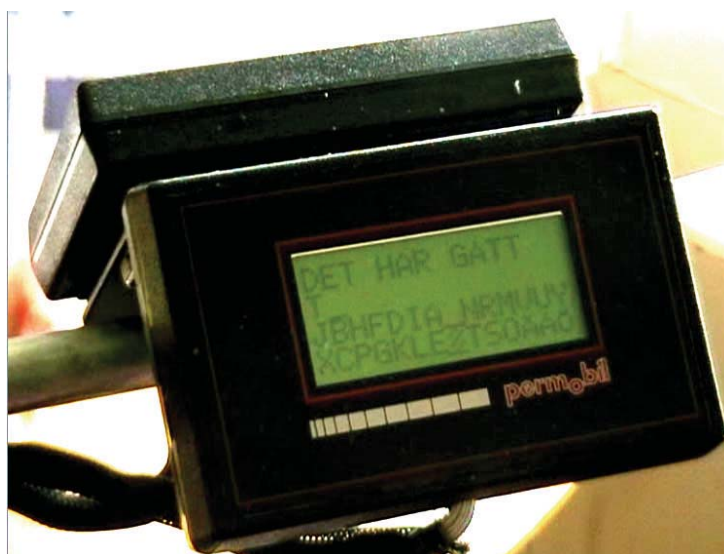
Figure 11.1. The Alfa Standard device with double displays and synthetic speech.
