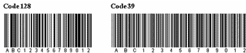
Figure 3-16: Comparison of symbol length between Code 128 and Code 39
