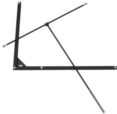
Figure 4. Reference object and wand used for dynamic calibration (with permission from Qualisys AB).
