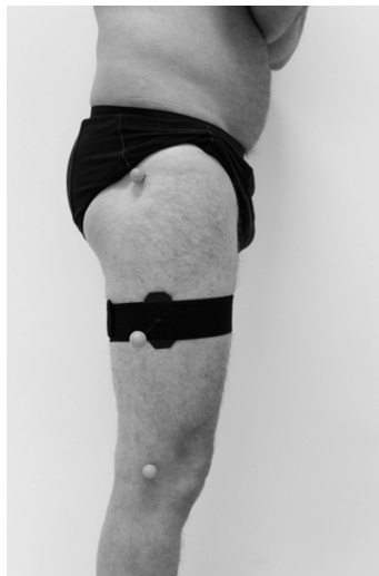
Figure 11. Subject with a wand marker on the thigh and skin markers on the great trochanter major and lateral side of the knee.
