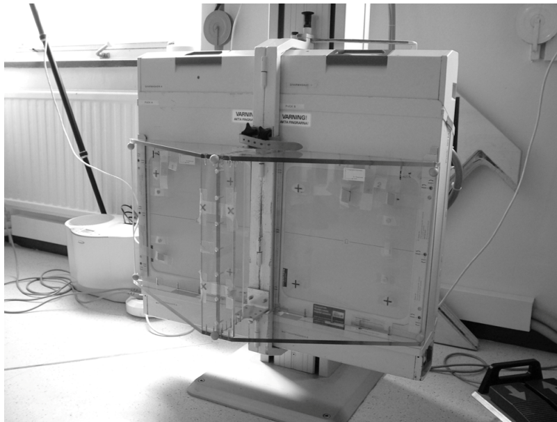
Figure 12. A uni-planar calibration frame mounted in front of the two film exchangers. In this case, the frame was equipped with six retro-reflective markers to make it possible to trace in the OTS.
