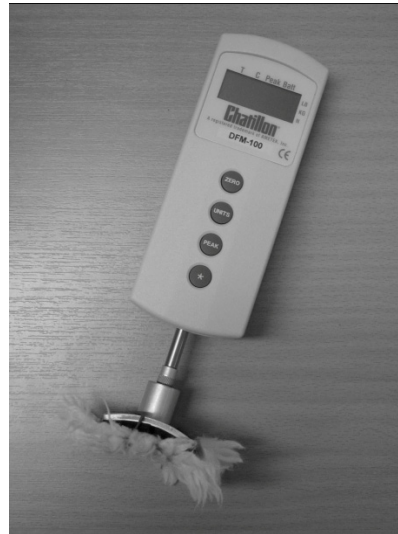
Figure 19. Hand held myometer used in study IV.
