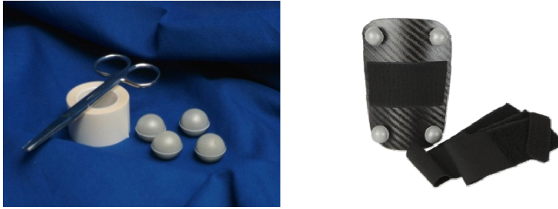
Figure 5. Skin markers and double-adhesive tape on the left, cluster markers with an elastic strap on the right (with permission from Qualisys AB).
