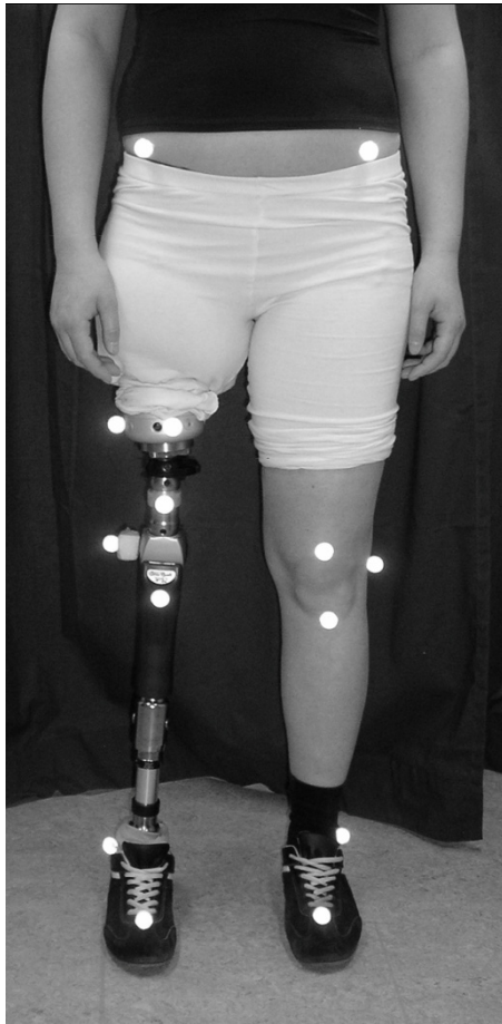
Figure 20. Patient with osseointegrated prosthesis equipped with reflective markers.
