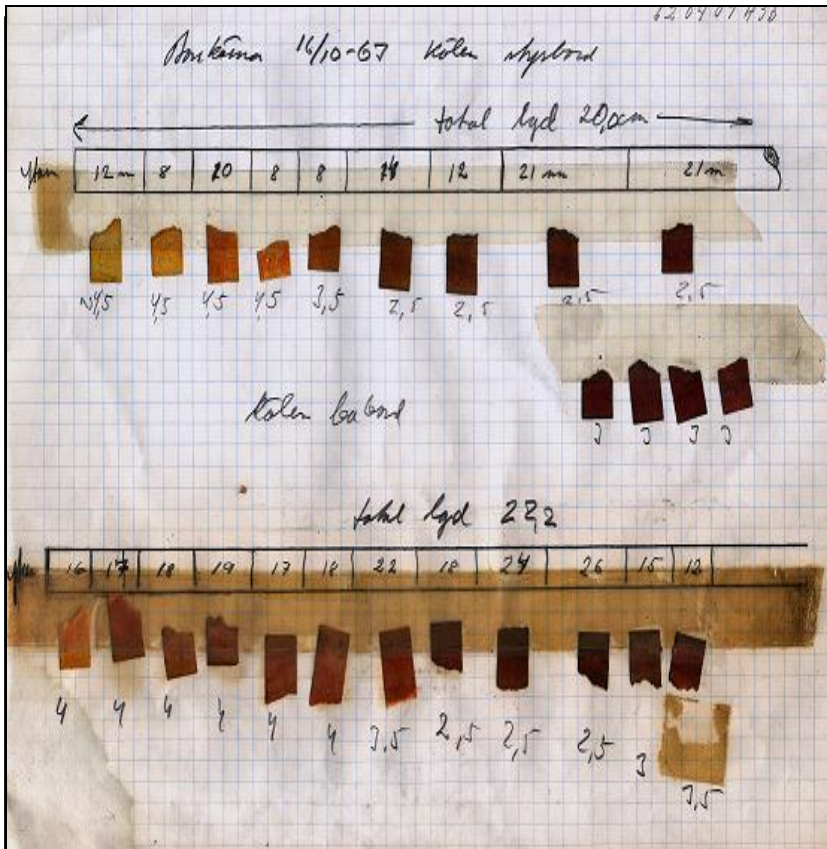
Figure 6-3. The liquid in each piece of two core samples from the keel of the Vasa was squeezed into pH test paper in a carpenter's bench. The pieces of pH test paper have been mounted on to a paper sheet with sketches of the wood cores and with the pH readings made at the time of the experiment. 165
