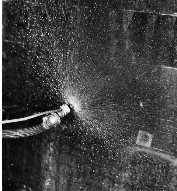
Figure 4-12 Area of delivery of outside spray (photo: Göran Sallstedt)
