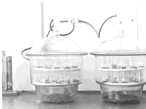
Figure 7-2 Drying the wood samples in vacuum chambers with silica gel (blue gel) (photo: Björn Hedin)
