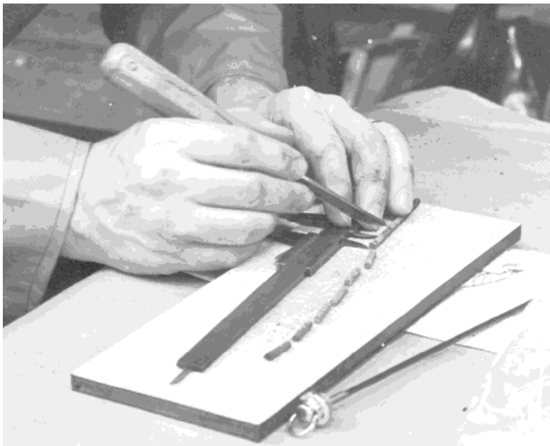
Figure 6-4 Cutting a wooden core from a heavy timber (photo: Sven Bengtsson)
