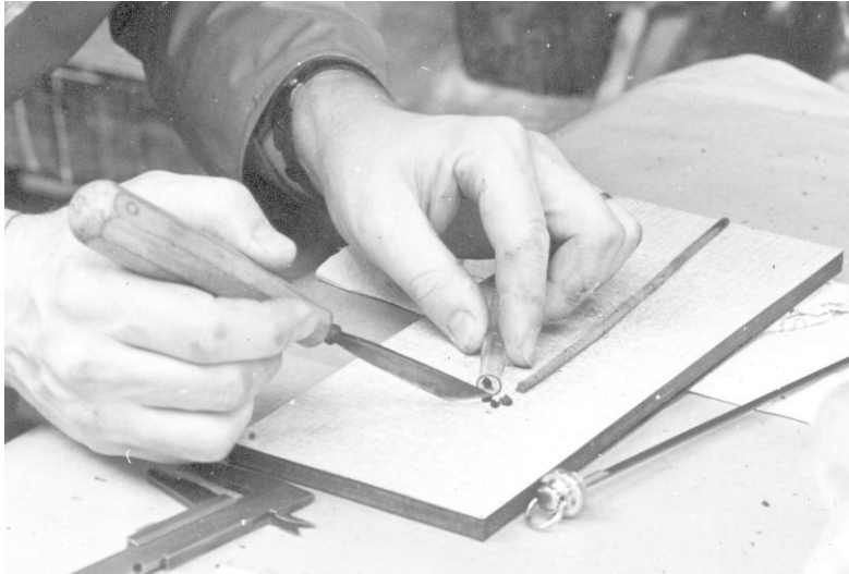
Figure 6-3 Putting the 10 mm surface layer cut from a wooden core into a specimen tube (photo: Sven Bengtsson)
