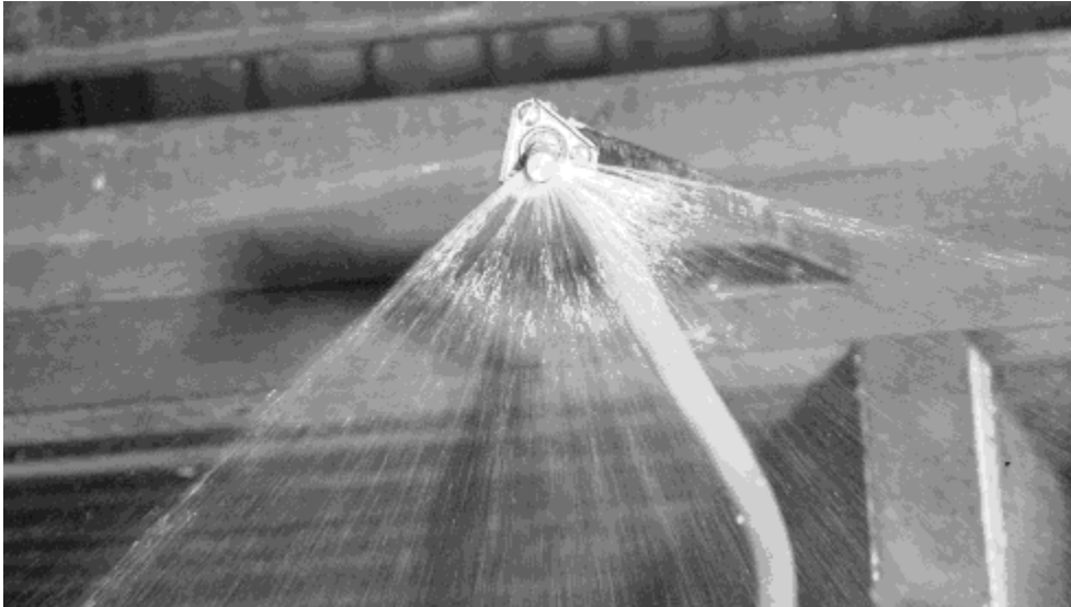
Figure 4-14 Delivery from spray nozzle into the space between the outside and the inside plankings (photo: Göran Sallstedt)
