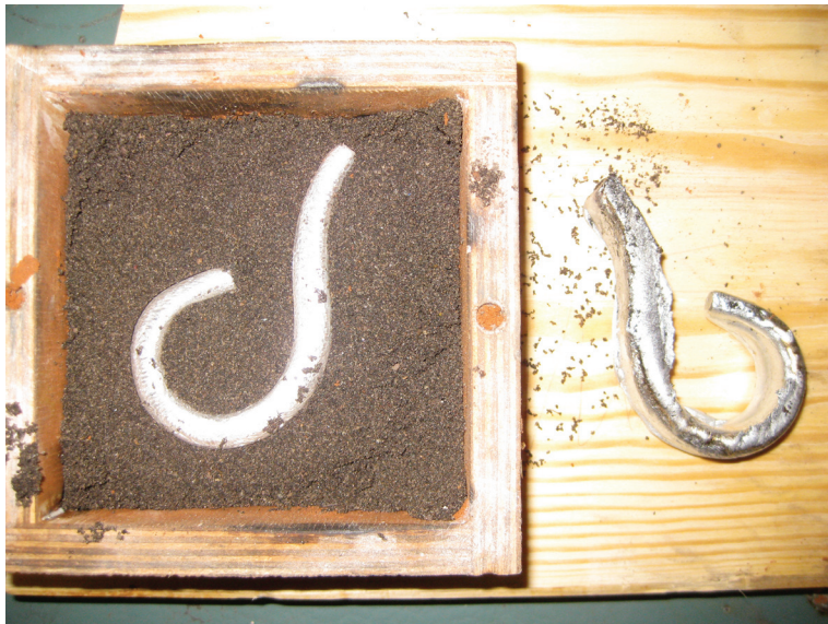
Below. Testing sand casting out of interest.
