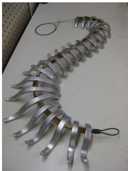
Right. Second half. After struggling with the first half I decided to profile the ends of each piece with a milling machine before bending. I had decided on the lengths of these pieces partly due to what material was left and how much longer the piece should be. Also the longer pieces took more time to form and finish and were heavier. At this stage there was still going to be a long tail.
