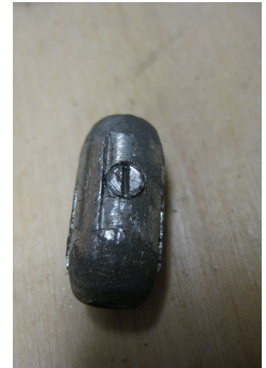
Above. A larger crimping tool for the 9mm aluminium spacers. I could not create enough force to crimp them so used a grub screw instead (right).
