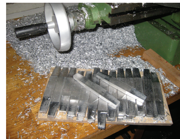
Right. Second half. After struggling with the first half I decided to profile the ends of each piece with a milling machine before bending. I had decided on the lengths of these pieces partly due to what material was left and how much longer the piece should be. Also the longer pieces took more time to form and finish and were heavier. At this stage there was still going to be a long tail.
