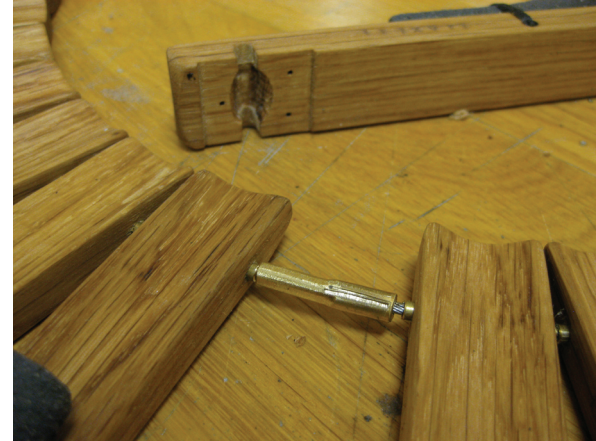
Above. The unfinished crimp joining the cable ends with the wooden piece to conceal it. A small brass cover conceals the crimp.
