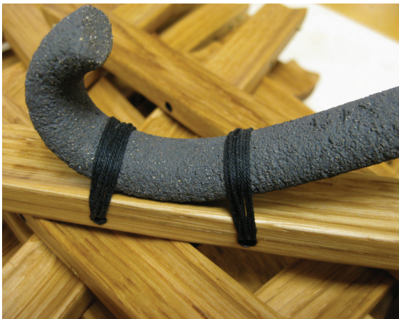
Left: Testing some string. This is cotton which I waxed. It was not strong enough so waxed polyester was used.
