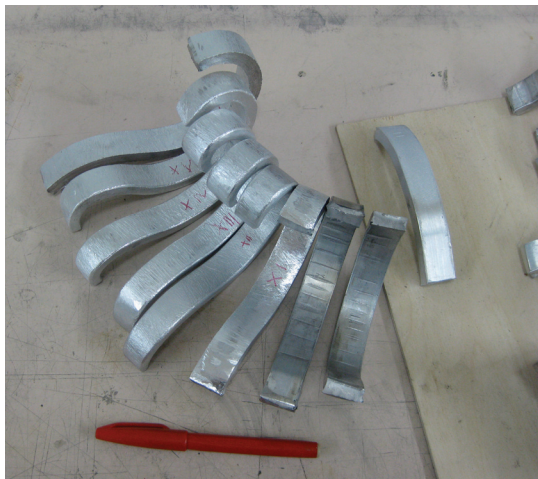
Left: Aluminium bar 20 x 10 mm hand forged to shape then filed to profile the ends.
