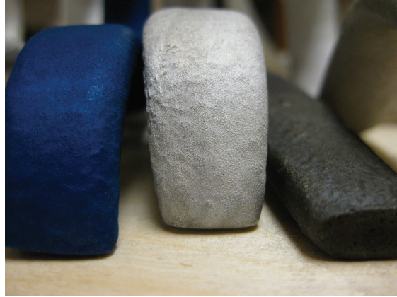
Above. The anodizing process and its results. I tried colour but preferred the light grey of un-dyed anodizing.
