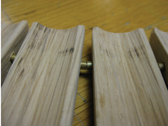
Left: The inner holes were lined with a brass tube which also acted as a spacer between sections.
