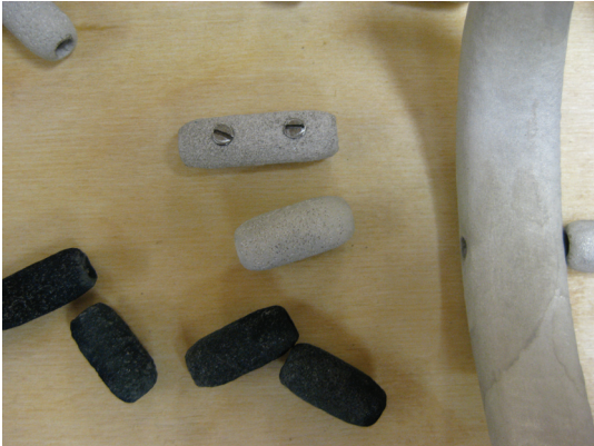
Left. The dark spacers were dyed black so they did not disturb the form at the crossing point.
