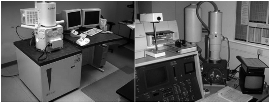
Figure 6. SEM instruments used in the thesis. Left: Philips SEM 515. Right: Gemini IMB LEO 1530 field emission SEM.
