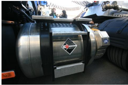
Figure 9, Tank for liquefied methane (picture: Sporer)
