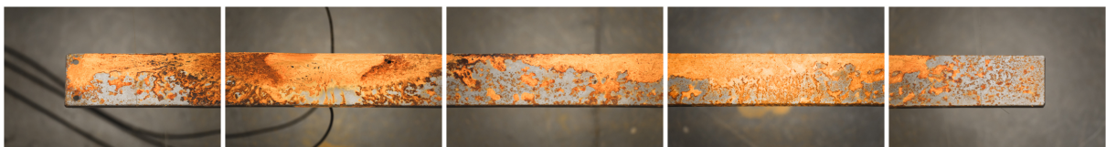
Illustration 16: The rust pattern on one of the bars
