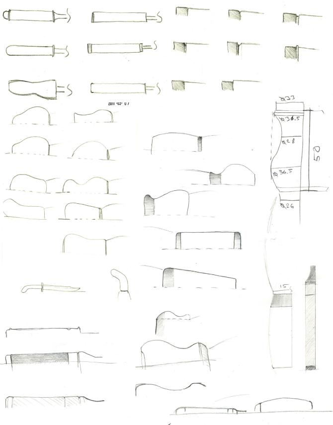
From that sketch phase a few ideas was chosen and tested in the shape of clay mock-ups. The goal here was to test sizes of the handle for the razor and the brush. The aim was to try out different shapes that both are usual but also new ways of handling the different tools.
