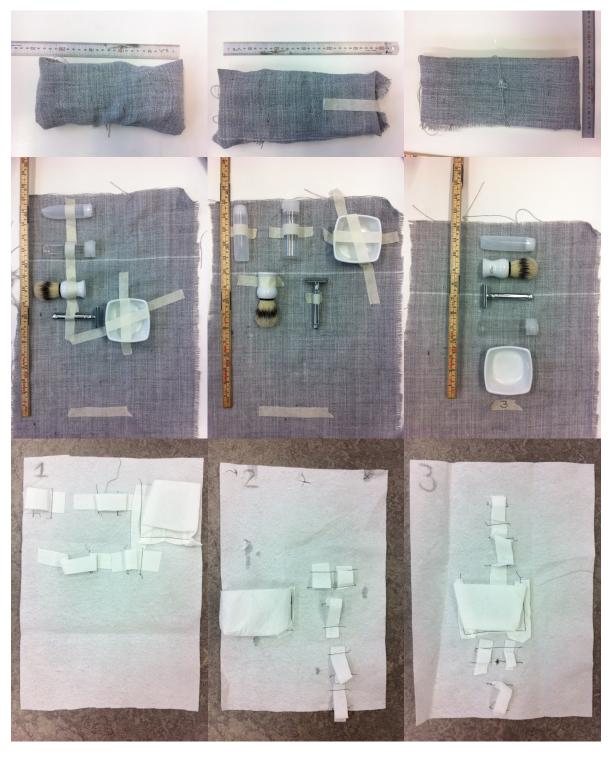
To make this picture even clearer illustrations of the different solutions was made to see how they could be perceived. From the mock-ups measurements the models was translated into illustrative pictures to get a feel for how the appearance could come to look. Below are different models of packaging, placing orders and folding techniques.
