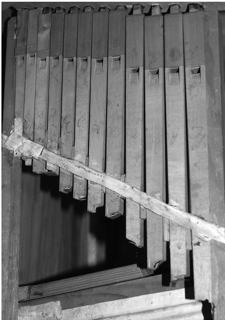
Figure 2.11: The treble rank of pipes is mounted upside down on the toeboard. In the top right of the picture are the feet of the lower rank of tenor pipes, mounted horizontally on the side of the toeboard. All of the pipe feet are glued into the toeboards.
