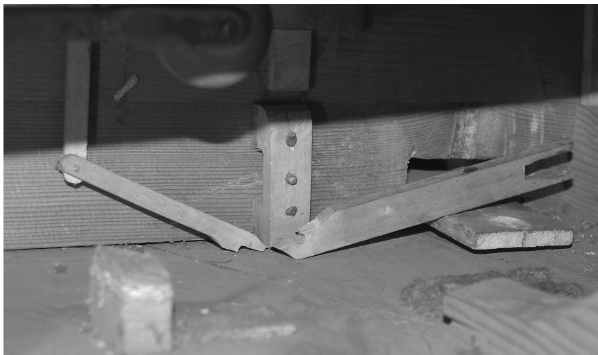
Figure 2.9: The lower part of the Windschweller mechanism. View from inside the case, facing the kneeboard. The back of the player’s left pedal is in the right bottom corner. It would have operated the backfall, now broken, lying on the floor.
