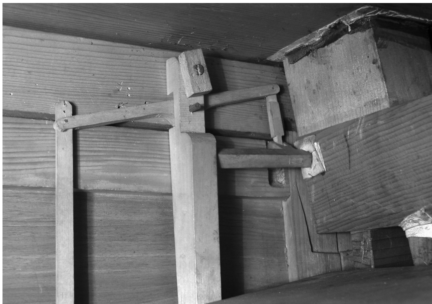
Figure 2.10: The upper part of the Windschweller mechanism. View from inside the case, facing the kneeboard.
