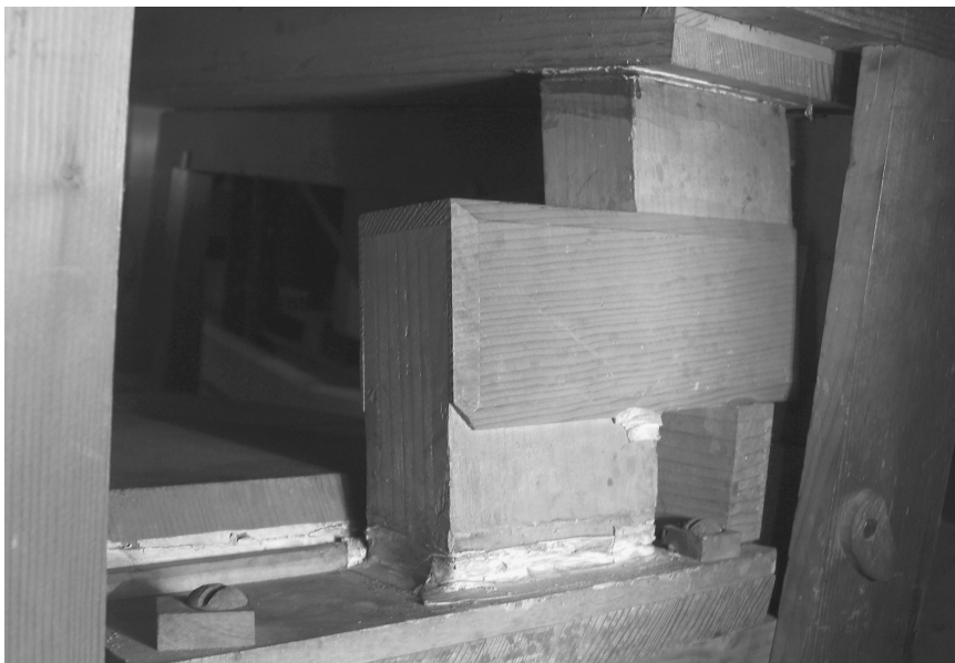
Figure 2.6: Bellows and wind trunk from the spine side.
