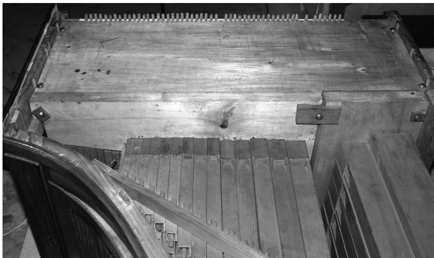
Figure 2.8: The top of the windchest with the toeboards mounted behind it. At the left of the picture are the feet of the treble pipes, racked upside down under the tenor toeboard.
