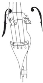
Screw to set the chinch to tailpiece and plug the cable to the pre-amp.
