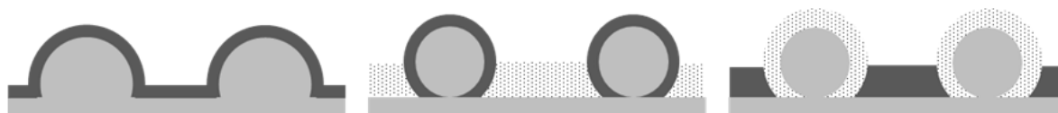
Figure 7.3 Schematic illustrations of the three types of nanopatterns that were created in the theses works. (Left) Surfaces with nanostructures and homogenous chemistry. (Center) Surfaces with adhesive particles and inert surroundings. (Right) Surfaces with inert particles and adhesive surroundings.
