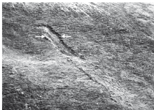
Figure 32. Example on shallow slide on top of the permafrost table in Adventdalen, Svalbard. The distance between the arrow is a few meter. Photo credit: Ernst Hauber
