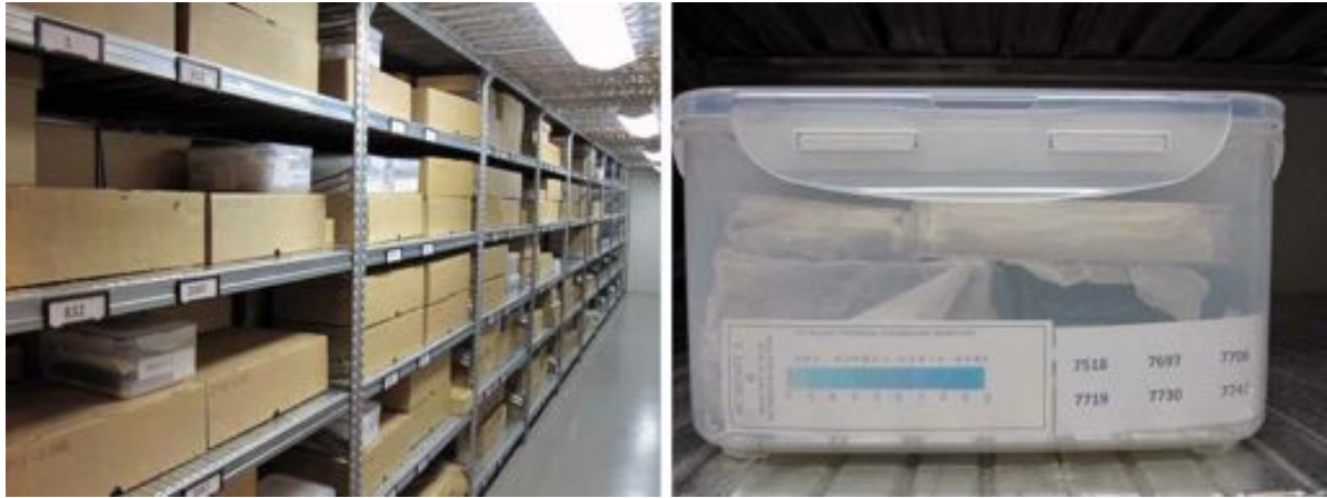
Figures 3 and 4. Aluminium shelves stacked with acid free cardboard boxes at the National Museum of Iceland. In between the cardboard boxes are PE boxes desiccated with silica gel for the storage of unstable artefacts. Figure 4 shows a close up of one those. Humidity strip and the numbers of the artefacts in the box can also be seen.
