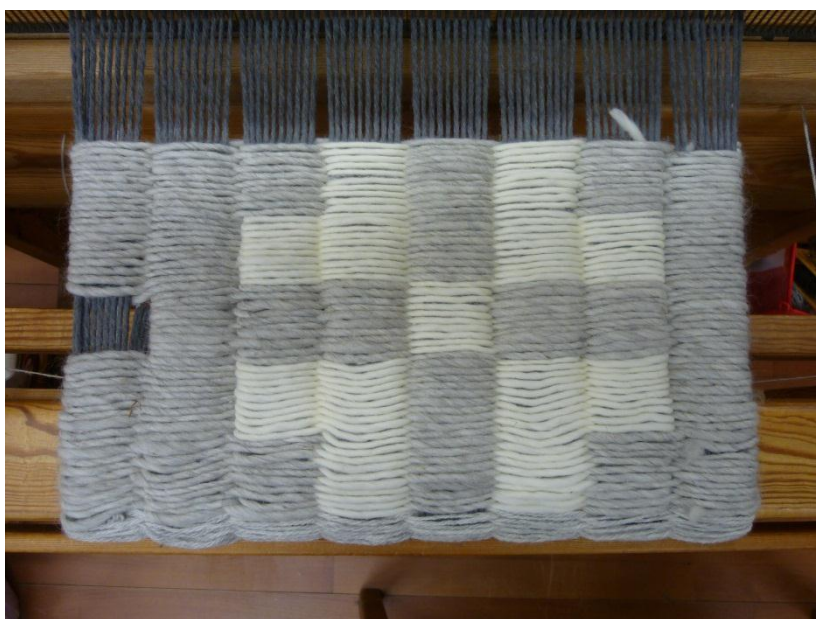
Test 3, width 48cm, material: warp: wool yarn, weft: wool yarn, December 2011
