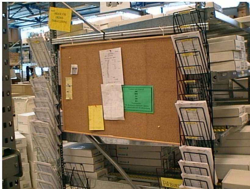
Figure 4: The board, without order lists. On the left-hand and right-hand sides are the paper tray columns used both by order packaging and product packaging for storing work orders.
