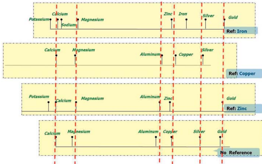
Diagram 5.5 Student-constructed electrochemical series lined up with reference to one metal (e.g., calcium)
