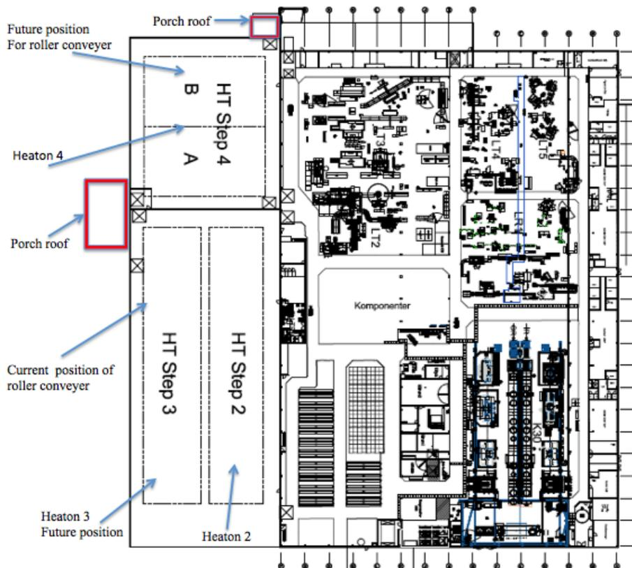
**Figure 6.7: Layout E-heat treatment, Source: SKF (modified)**
