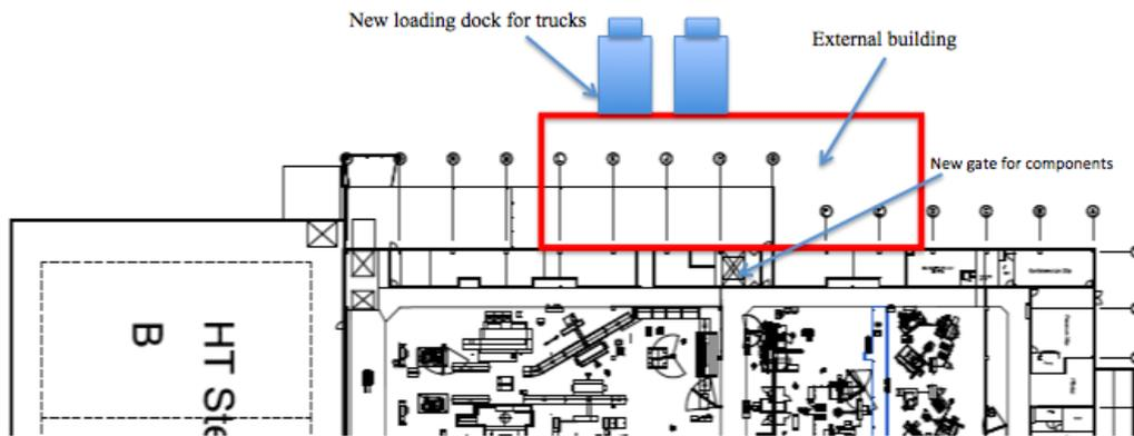
**Figure 6.5: New external intermediate storage area, Source: SKF (modified)**
