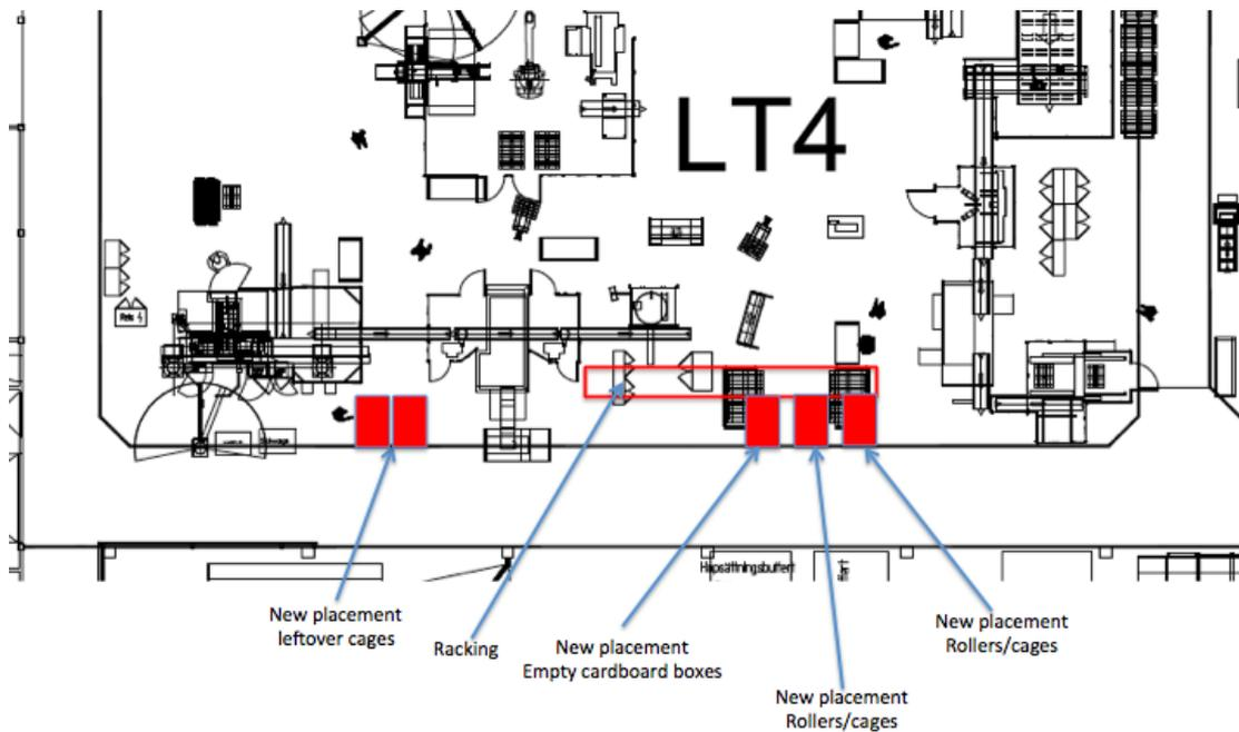
Figure 6.17: New layout end of channel LT4, Source: SKF (modified)
