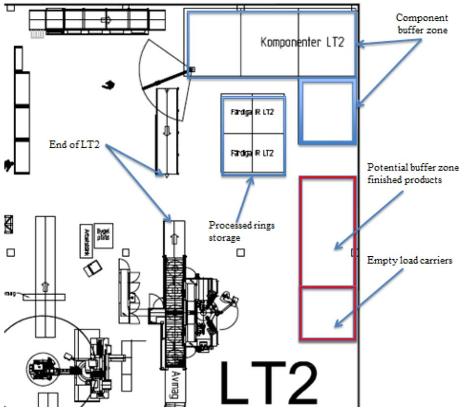
Figure 6.23: End of channel LT2, Source: SKF (modified)
