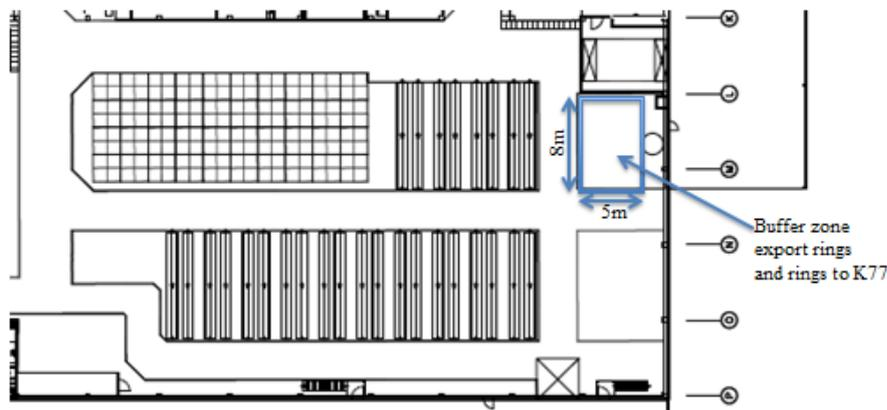
Figure 6.10: Buffer zone export rings, Source; SKF (modified)
