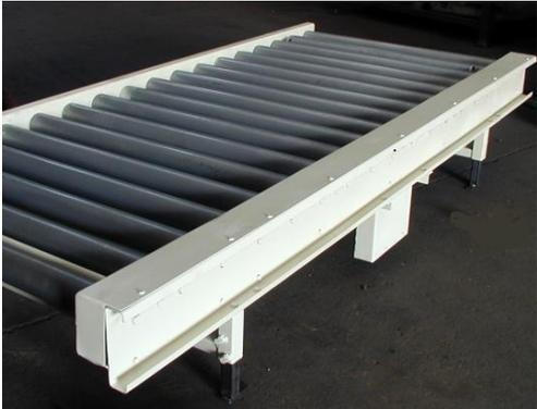
**Figure 3.1: Roller Conveyor, Source: [www.asconveyorsystems.co.uk](http://www.asconveyorsystems.co.uk)**
