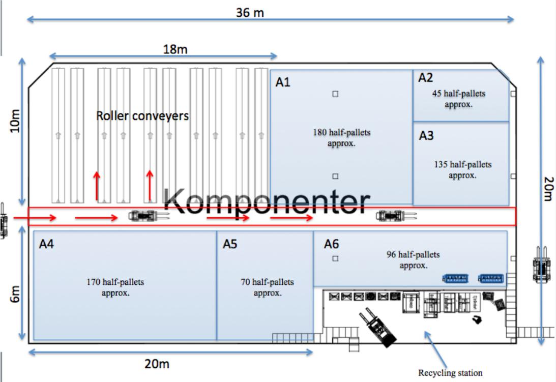
Figure 6.11: Intermediate component storage, Source: SKF (modified)
