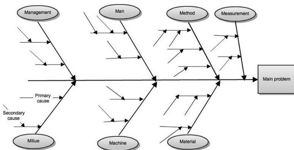
Figure 3.9: 7M-diagram, Source: Bergman and Klefsjö, 2008
