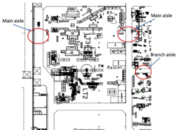
Figure 6.2: Main and branch aisles in the E-factory, Source: SKF (modified)
