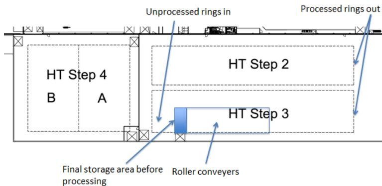
Figure 6.9: Buffer zones E-heat treatment, Source: SKF (modified)
