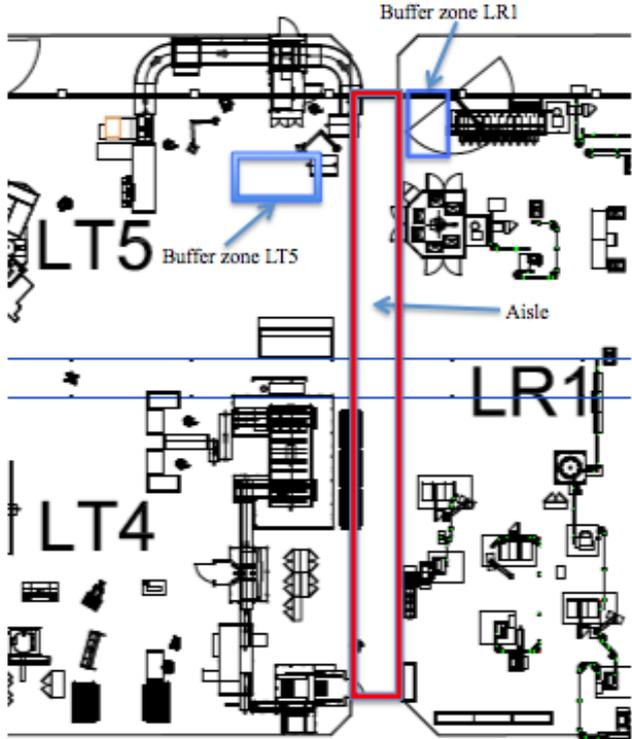
Figure 6.3: Aisle between LR1 and LT5, Source: SKF (modified)
