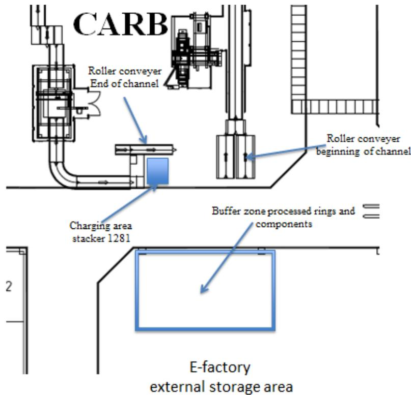
Figure 6.24: Beginning of channel CARB, Source: SKF (modified)
