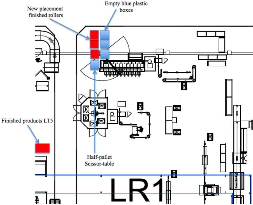
Figure 6.29: New layout end of channel LR1, Source: SKF (modified)
