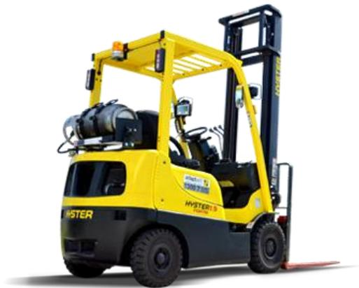
**Figure 3.5: Counter Balanced Truck, Source: [www.usedforklifts.com](http://www.usedforklifts.com)**
