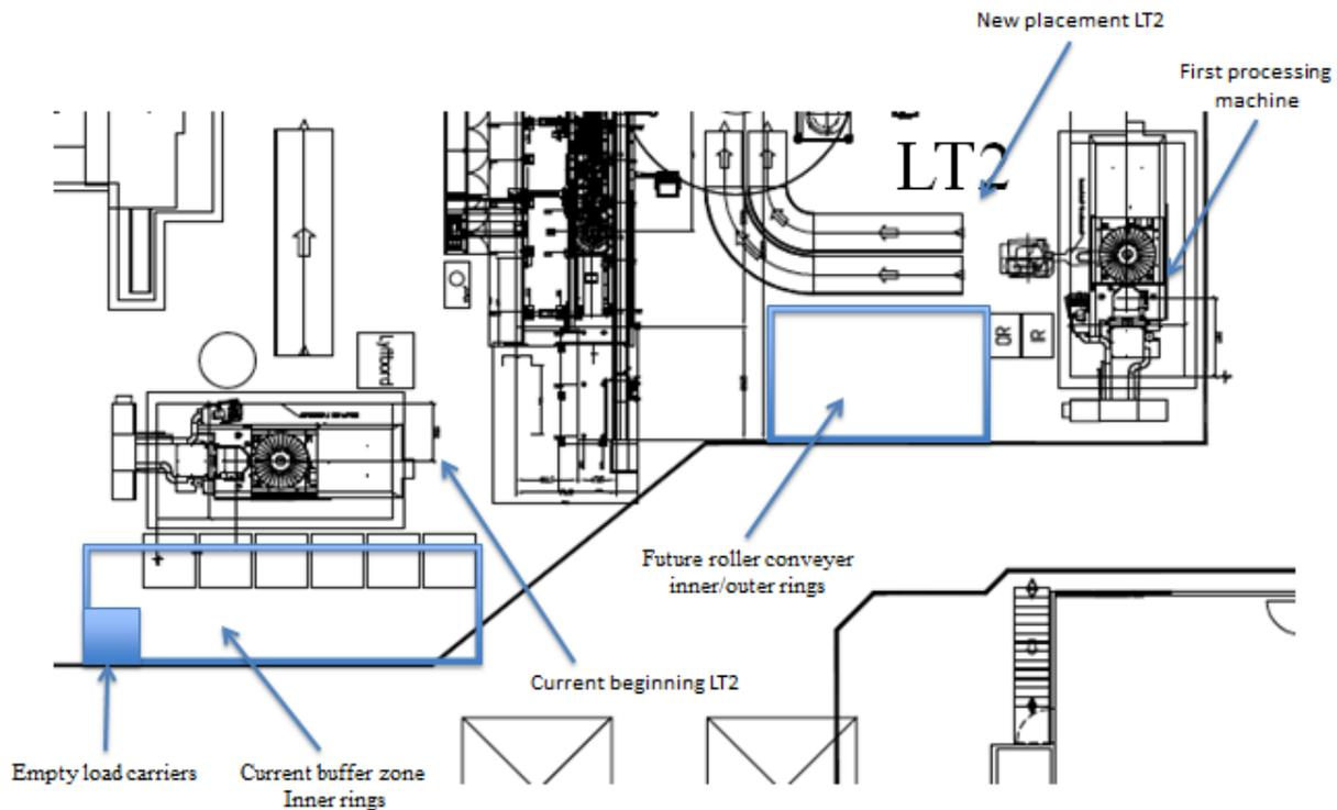
**Figure 6.22: Beginning of channel LT2, Source: SKF (modified)**
