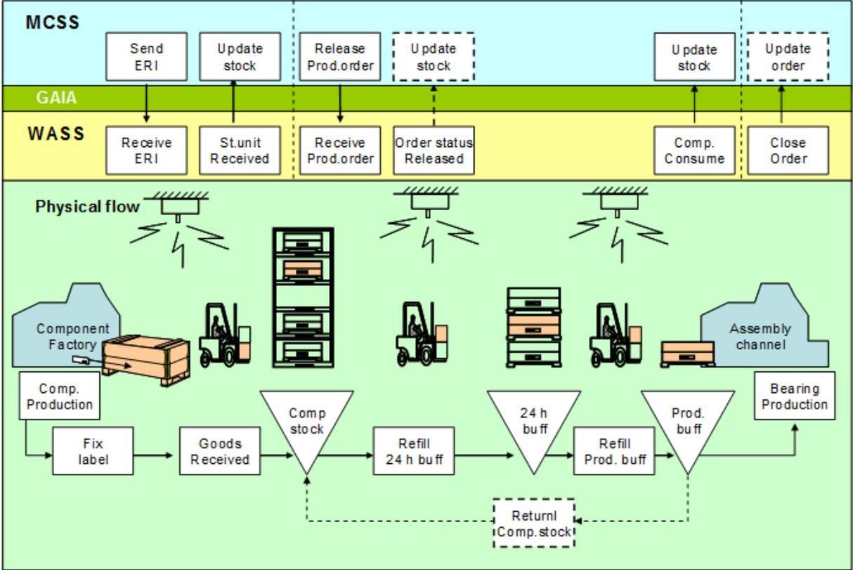
Figure 6.30: Information flow for use of WASS, Source: SKF
