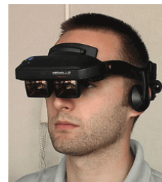
Figure 1: Video see-through HMD that includes cameras for capturing the real-world scene
