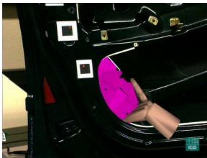
Figure 3: Real world scene with superimposed 3D model that was designed in the production stage. The scene is a moving instruction for that particular part. (Reiners, et al., 1998)
