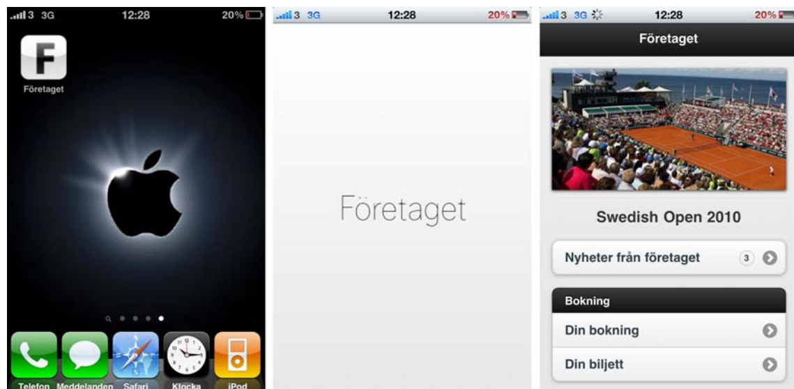
Figure 44. Showing how Företaget has been added to the home screen of the iPhone, then in the middle picture we see a splash-screen as the site loads and in the third picture we see how there is no address bar on top and no navigational buttons in the bottom area of the site.
