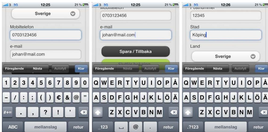
Figure 23. Three different types of optimized keyboards for the specific content type. Keyboard for entering mobile phone number to the left, optimized for e-mail in the middle and to the right only letters are shown for writing the name of a city.
