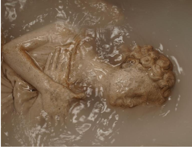
Figure 1- Barium hydroxide method, Limestone, photo; Vinka Marinkovic 2011
