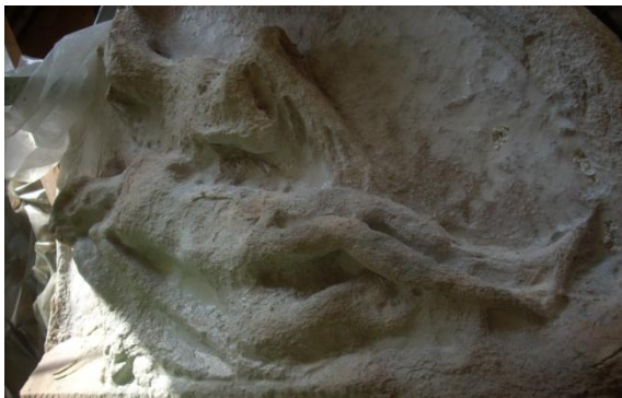
Figure 10- The moment relief was taken out of Ba(OH) 2 solution
