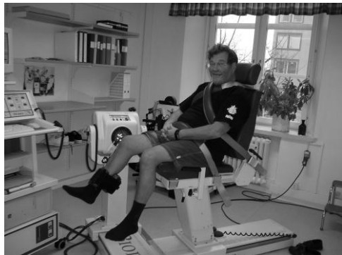
Figure 2: Isokinetic knee muscle strength measurement, performed in a Biodex dynamometer (the subject gave his permission to publish the picture).
