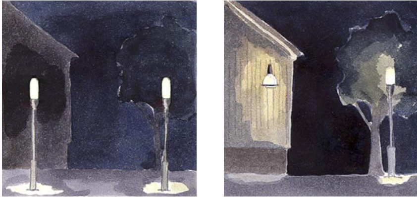
Figure 2. When these luminaires are placed closer to the facade and the tree, more of the light is seen and the surrounding contrasts become softer, reducing the risk of glare.
