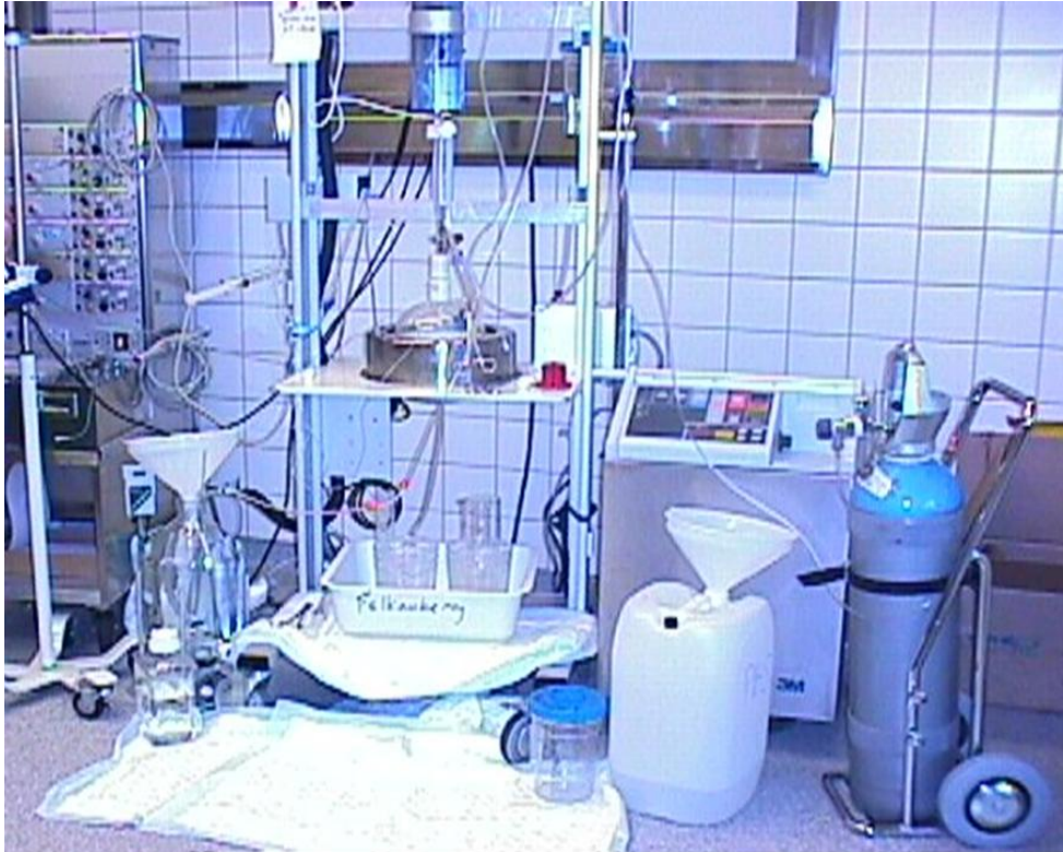
Figure 20. Langendorff perfusion. To the left the polygraph, in the middle the Langendorff perfusion device, and to the right the heat exchanger from a cardiopulmonary bypass machine.
