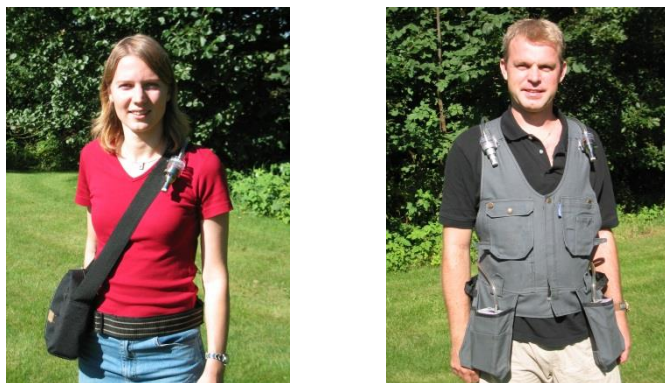
Figure 1. (a) Personal sampling equipment for PM_{2.5} (b) Duplicate personal sampling equipment ( PM_{2.5} and PM_1 )
