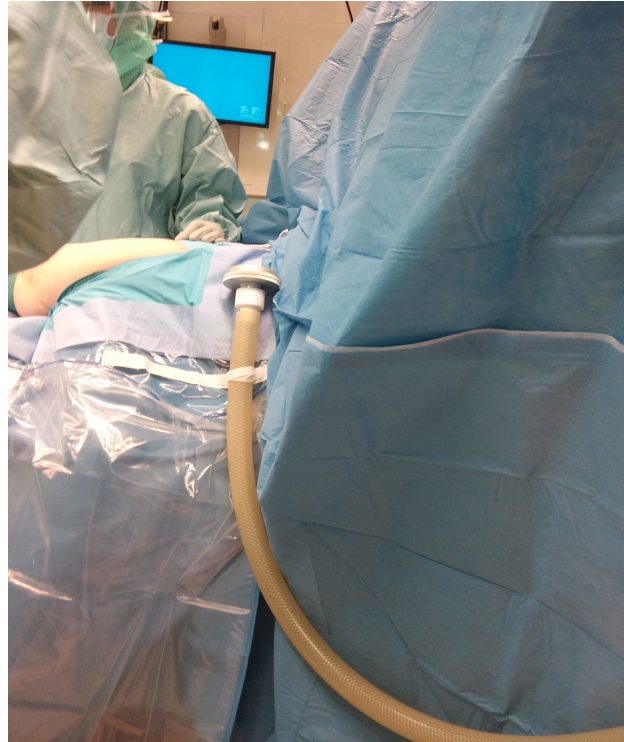
Figure 7. The air sampling hose with attached filter just before incision. Photo by Annette E Andersson.
