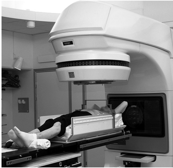
FIGURE 3.1. Patient in the stereotactic body frame at the Sahlgrenska University Hospital. The patient is immobilized using a vacuum pillow and the body frame is placed relative to the treatment machine using designated rulers.
