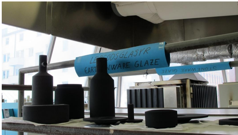
Colored and glazed with black and cobalt and waiting for the final firing
